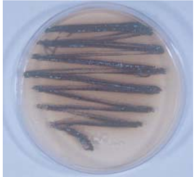
Figure 6. A colony of a melanin-producing fungus isolated from a rock surface and transferred to the laboratory in order to imitate natural bio-patination processes.
